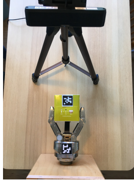
Fig. 2 Setup for collecting data. Two fingers of the SDH hand are used to grasp an object. The Asus Xtion PRO camera tracks the marker positions continuously during grasp attempts.
